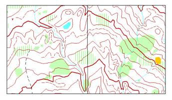
The best "O" maps are made from aerial photographs. The airplane is flown at an altitude about 10,000 feet above the terrain so that the scale of the images on the 9" X 9" negative is about 1:12, 000. The exposure interval is such that 60% of the land below that appears on a negative will also appear on the next negative. This is called overlap. Flight lines are flown so that there is overlap on the sides, too, called sidelap.
